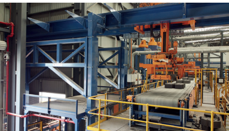
Top view of cuber pos. 251 with belt conveyor for infeed to splitting line
