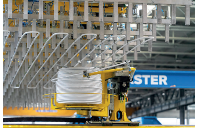
The Tube Master was specially developed by the Progress Group for bending and installation of tubes within precast concrete element production.
