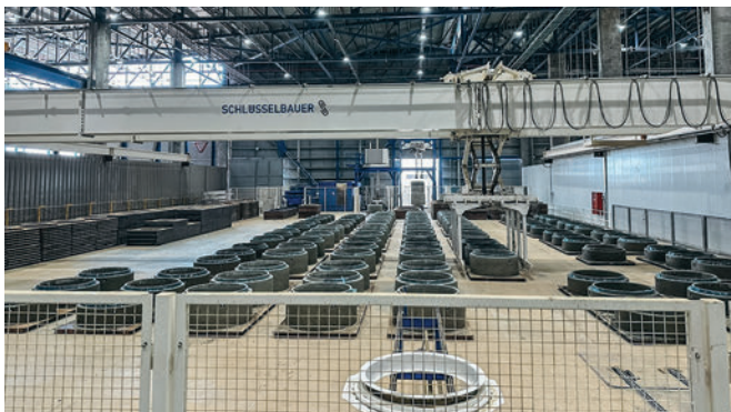
The curing area for standardized manhole risers with the Transexact automatic crane.
