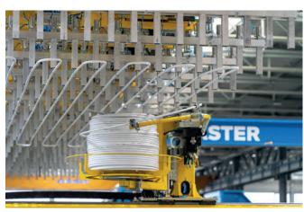
The Tube Master was specially developed by the Progress Group for bending and installation of tubes within precast concrete element production.
