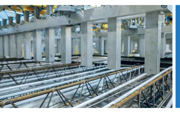
The system can lay pipes directly on the already inserted reinforcement and replaces tedious manual work.
