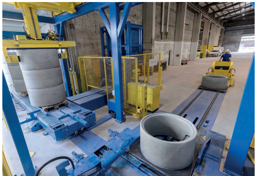
Manhole rings up to DN1500 are produced on the Magic 1501, first installed in 2021, as reported in detail in CPI 01/2022.
