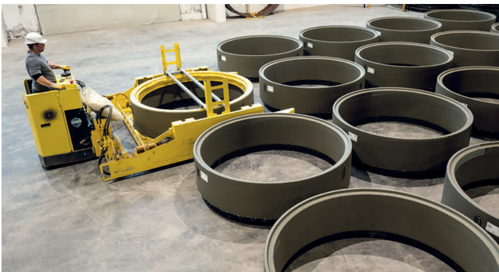
Fresh products are carefully transported to the curing area using an electrical cart for transportation and a set ring manipulator.
