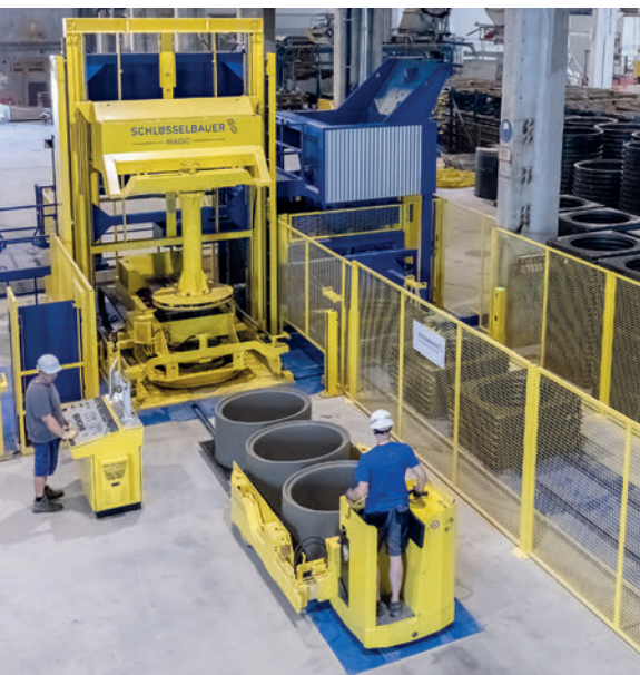
Manhole rings up to DN1500 are produced on the Magic 1501, first installed in 2021, as reported in detail in CPI 01/2022.
