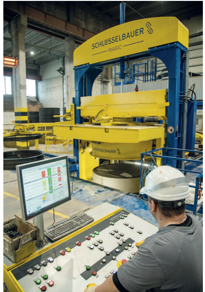
In order to ensure the fresh product is demoulded carefully, the mould and the press unit are raised in cycles.
