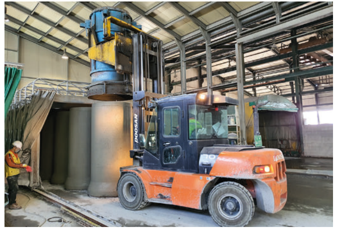
Professional production of concrete pipes DN 1000
