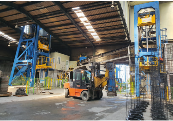
Preparation for concrete pipe production
