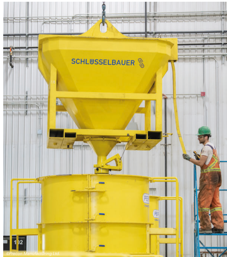
The mobile concrete silo can be operated using a hall crane or forklift.
