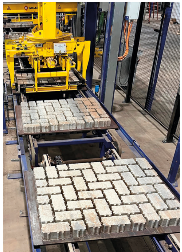
Masa's electro driven cuboter precisely places the layers on a conveying system and creates accurate cubes without damaging the products.
