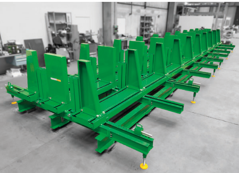
The double moulds are being used for producing the best-selling products - the columns and are 14 meters long.
