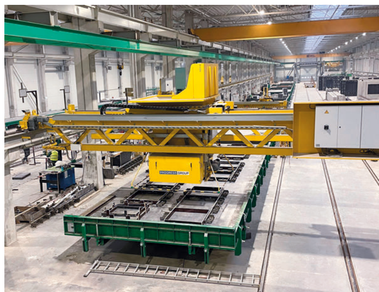
The concrete delivery system flying over the pallets is handling the delivery fully automated and with exact data, thus is saving concrete and time.
