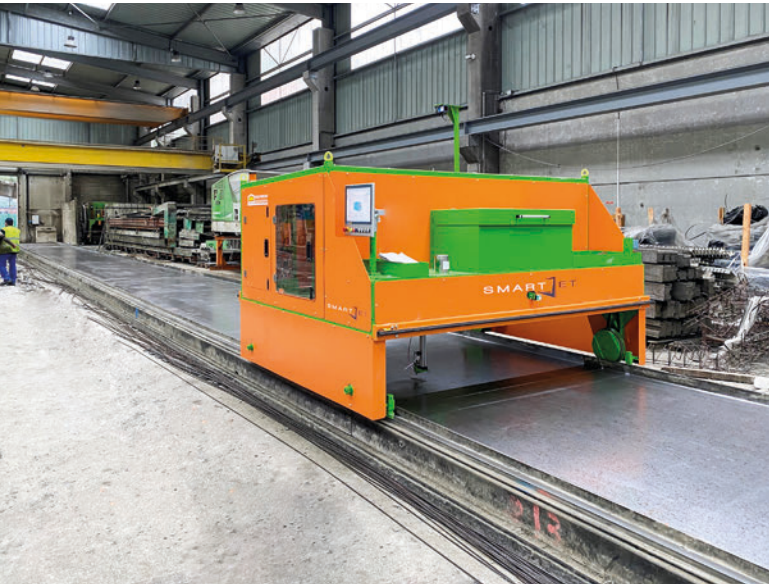
Since the automatic plotter is battery-driven, no cabling is required.
