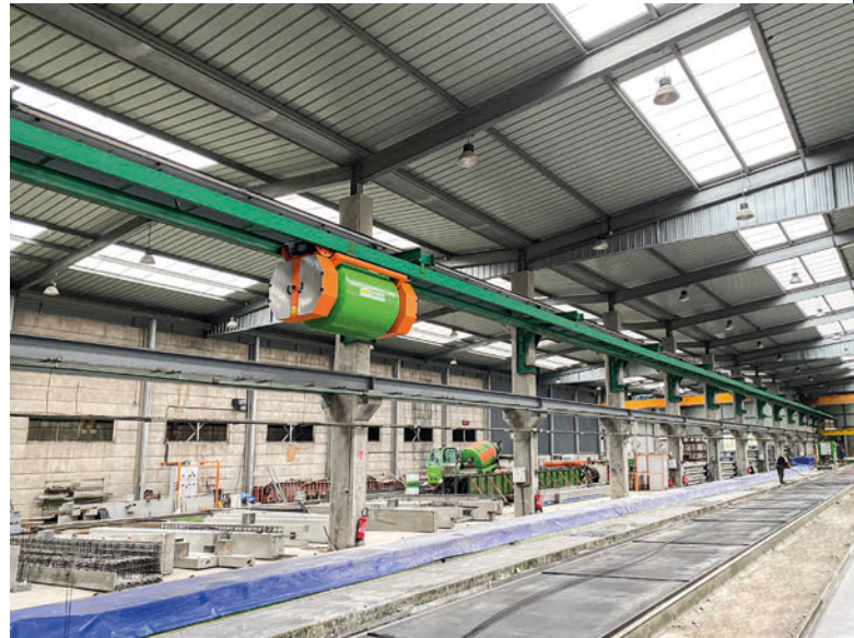
The flying bucket D-Flyer transports dry or wet concrete from the concrete mixer to the designated position in the production facility on elevated tracks.
