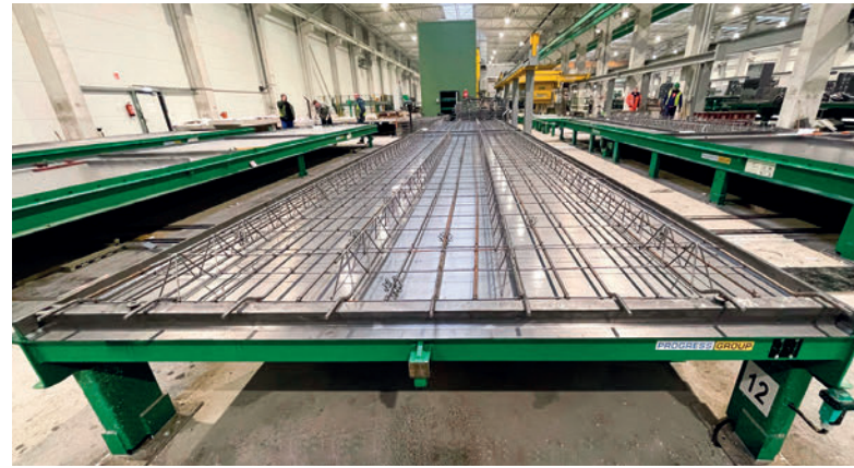
The reinforcement for the elements is being produced automated and thus exactly as planned.
