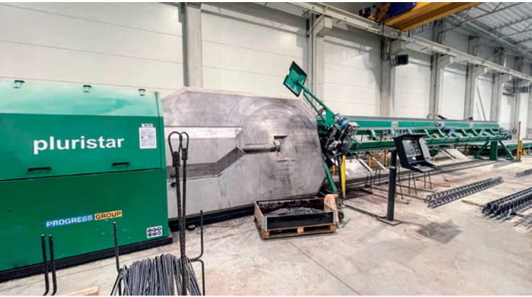
The multifunctioning machinery Pluristar can straighten, cut and bend the needed reinforcement steel directly from coil.
