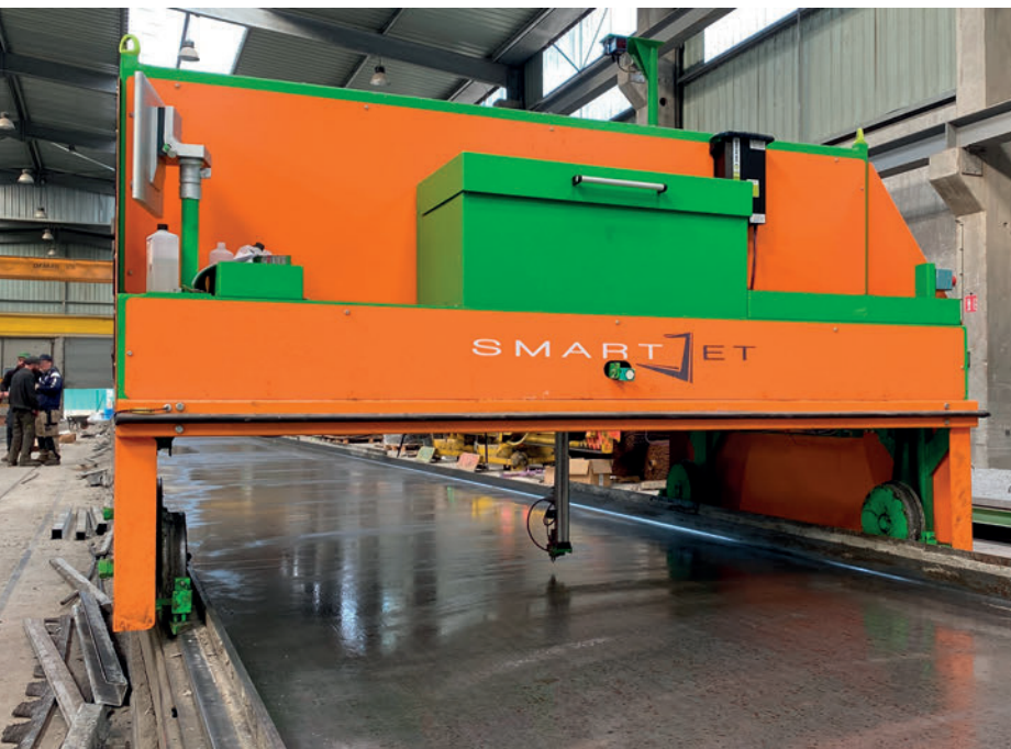
The automatic plotter SmartJet makes it possible to draw data such as inserts, shuttering placements and cutouts.
