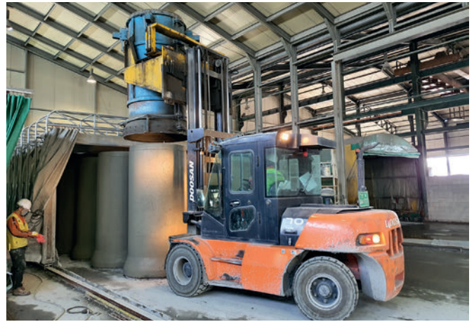
Professional production of concrete pipes DN 1000
