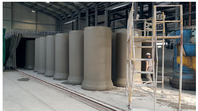
Freshly produced concrete pipes DN 1000 with integrated gasket
