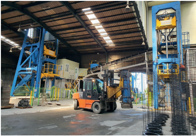
Preparation for concrete pipe production
