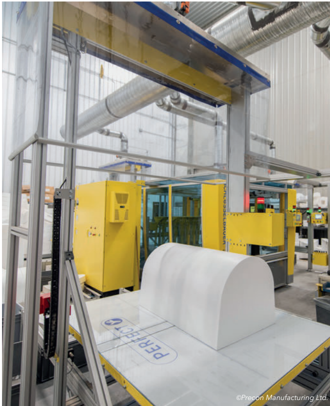
In channel production, a custom moulded body is created with just a few cuts and hand movements.
