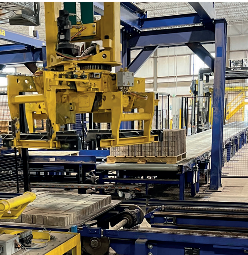
Masa's electro driven cuboter precisely places the layers on a conveying system and creates accurate cubes without damaging the products.
