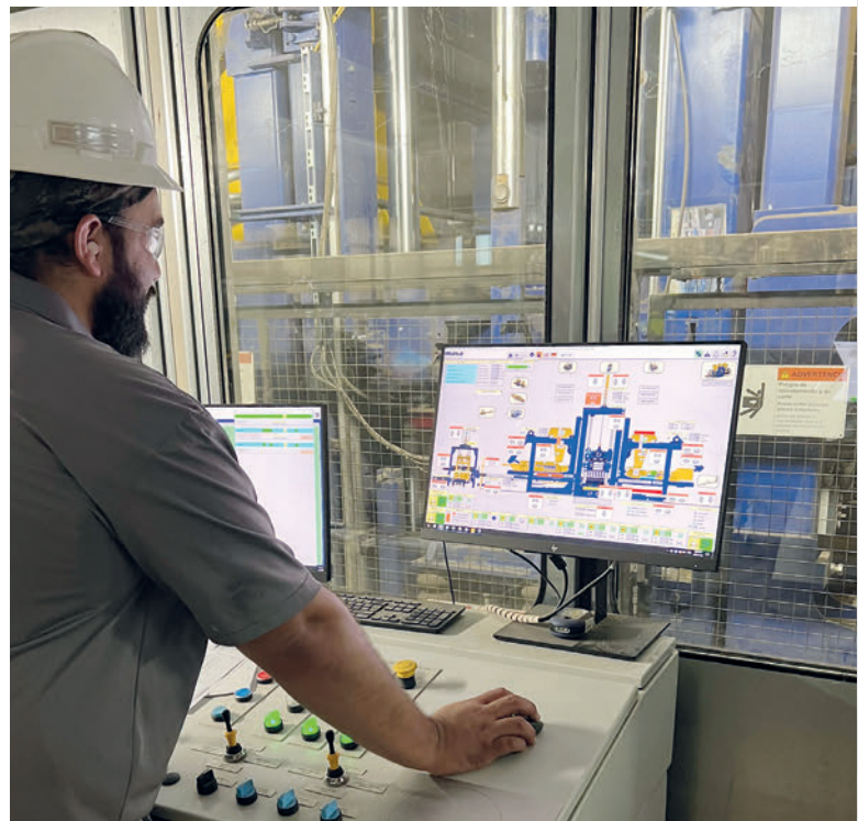
Real time animated controls allow the operator to see all processes at any stage from multiple screens.
