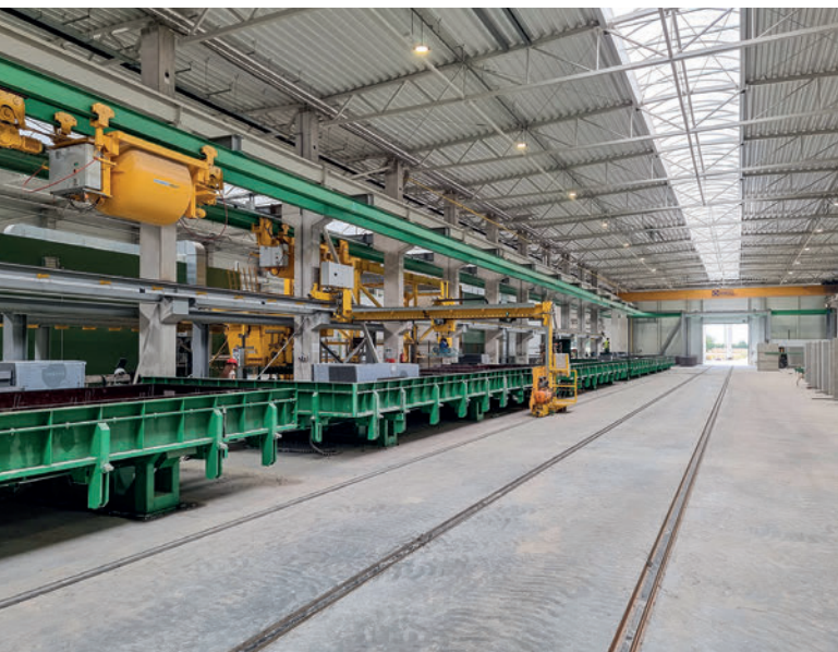
The tilting tables are used for the production of large area flat precast concrete elements, such as solid walls or sandwich walls.
