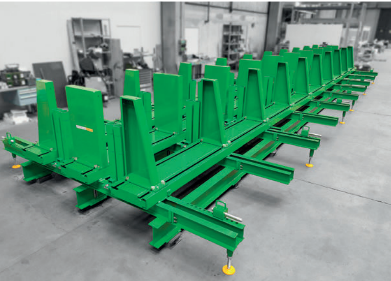
The double moulds are being used for producing the best-selling products - the columns and are 14 meters long.
