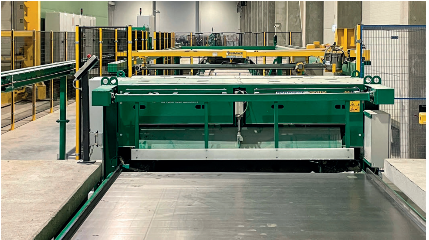
Before entering the system again, the pallets are being cleaned automatically.
