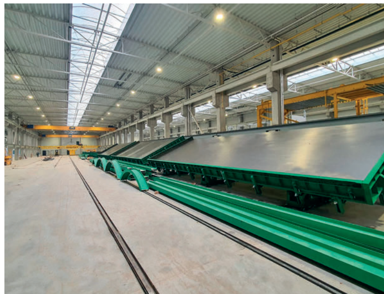
The tilting tables are used for the production of large area flat precast concrete elements, such as solid walls or sandwich walls.
