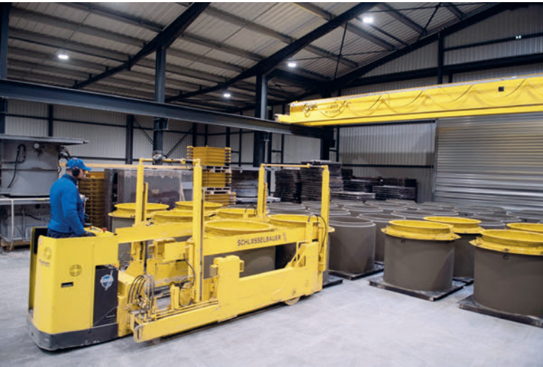
Products are transported to the curing area and on to the palletizing system using one of the three electrical carts for transportation.
