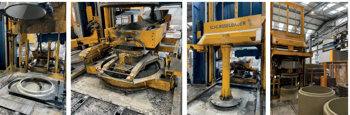
Manhole riser production with the Magic 1
