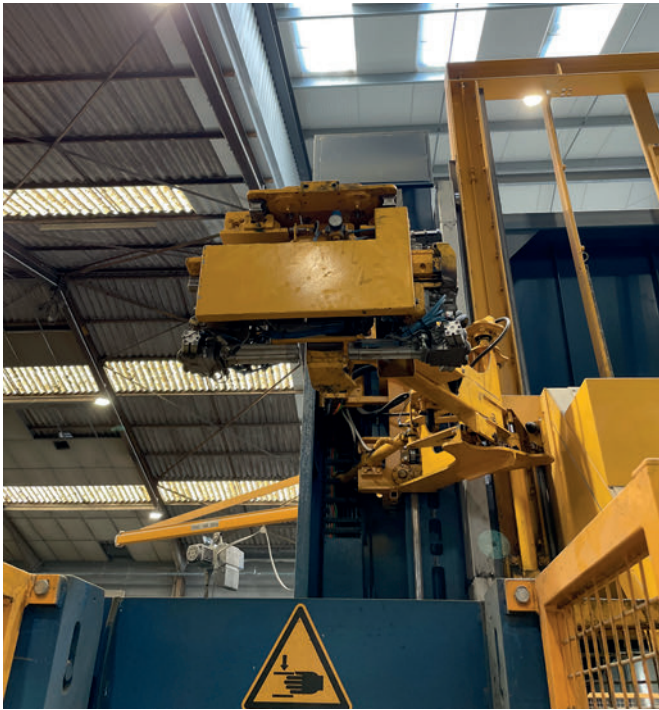
The Magic 1 automatic anchor robot
