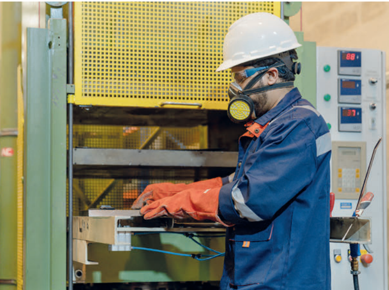
Rubber matrice production for customized concrete slabs in the Topwerk Middle East office in Dubai
