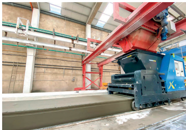
With the new machinery they can produce high-quality hollow core slabs, while also guaranteeing a high degree of fire resistance.
