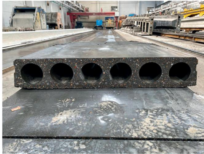
High surface quality of the hollow core slab is achieved easier with a highly automated machinery park.
