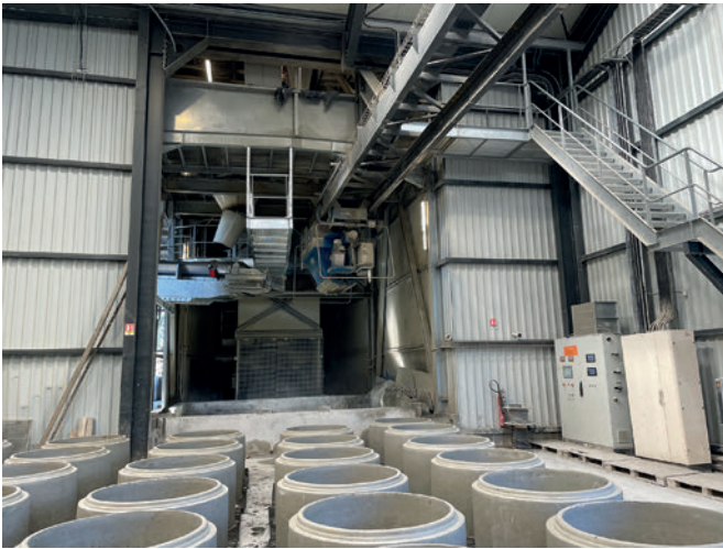
The Teka mixing plant produces the concrete for all the production areas
