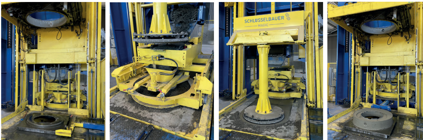
Fully automatic production of manhole covers with the Magic 2
