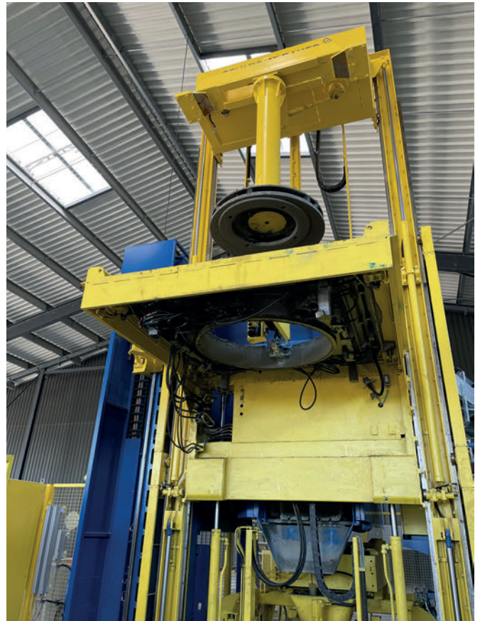
With the Magic 2, transport anchors are also inserted automatically
