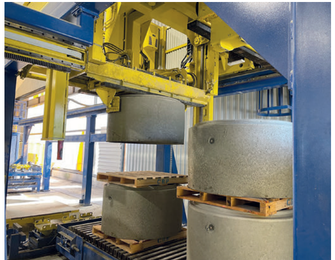
Palletizing of manhole risers
