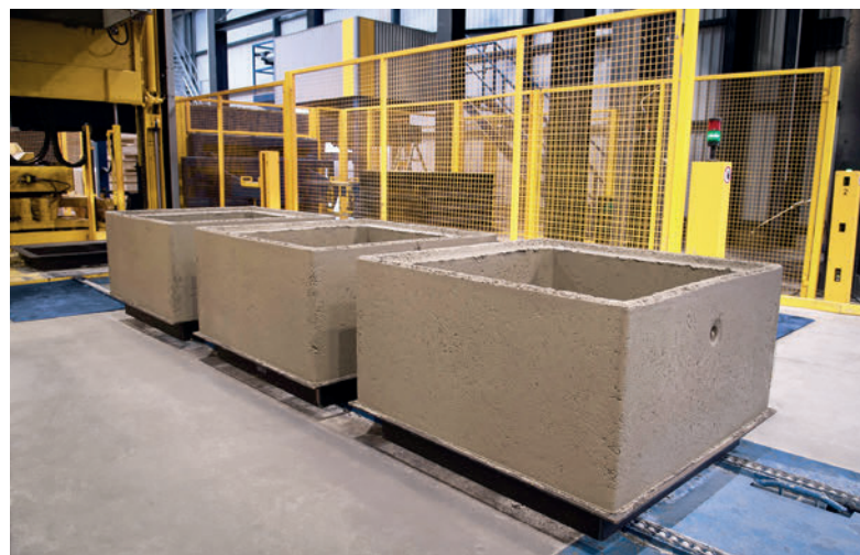
CRP SAS uses the Magic1501 to manufacture both square and round manhole components in a range of product heights
