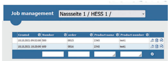
The order management in the Professional module enables the plant operator to record the planned products, the times, and the produced quantities according to the order.
