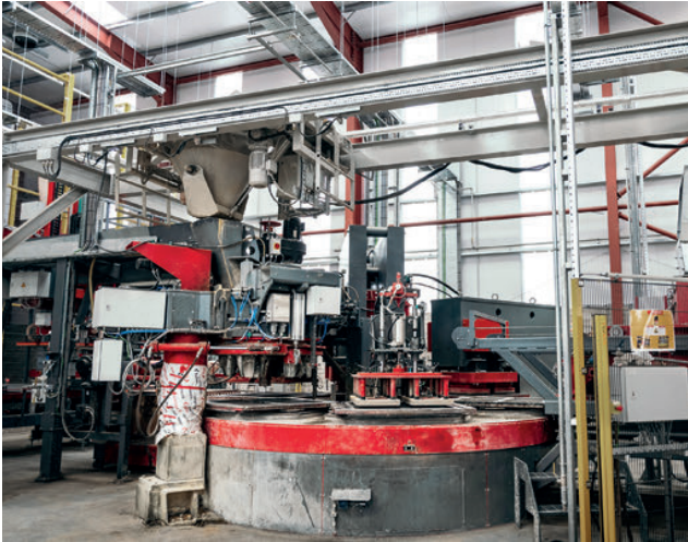
Tobermore opted for the UNI 1200/6 hermetic press with six working stations to produce double-layer concrete slabs.
