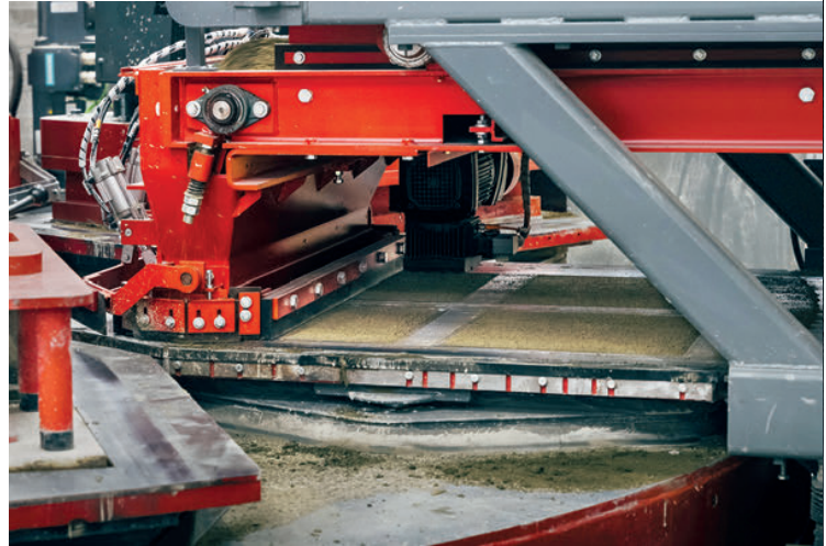
Tobermore opted for the UNI 1200/6 hermetic press with six working stations to produce double-layer concrete slabs.
