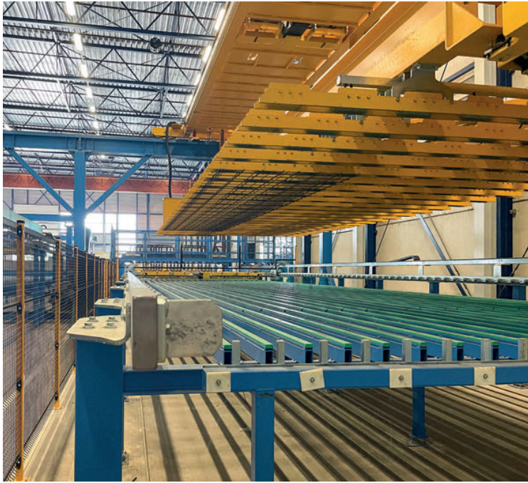
A magnetic crossbeam transports the meshes and cages fully automatically to the next station
