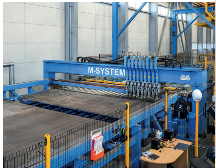
The M-System mesh welding plant is providing a high output with very high flexibility and automation and is producing directly from coil.
