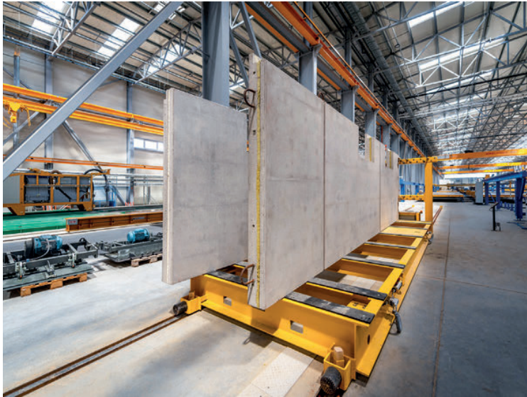
The finished prefabricated concrete walls and slabs can be produced under any weather condition and thus ensure a secure planning of the building.
