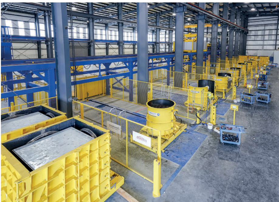
Several set-up locations for wet cast moulds ensure that there are no delays in the overall system despite varying set-up times.
