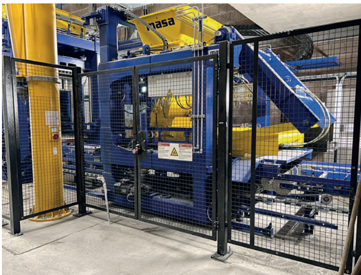
Masa XL 9.1 with column-mounted slewing grab
