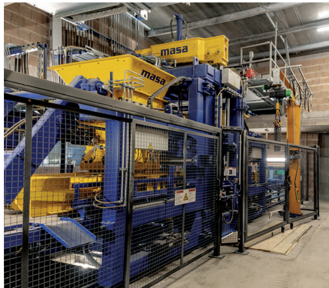
The new Masa XL 9.1 with decoupled column-mounted slewing mold change grab
