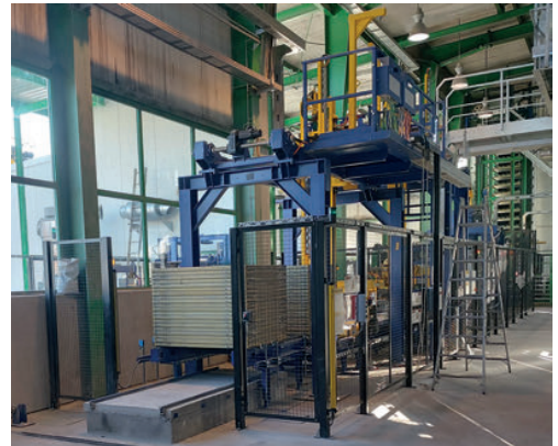
The new storage area offers space on several floors for the flexible temporary storage of up to 1,560 production boards
