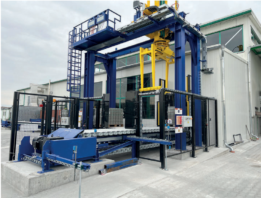
The cube shifter grabs the finished cubes with a special clamp and positions them
