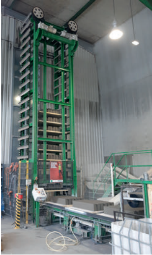
The stacks of production boards are well prepared and transferred to the storage area
