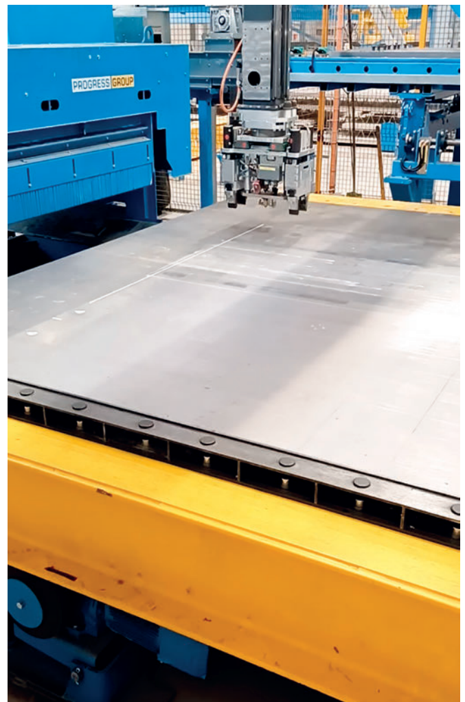
The marker for the placement of the shutters are made precisely with the help of the integrated software and fine lasers.
