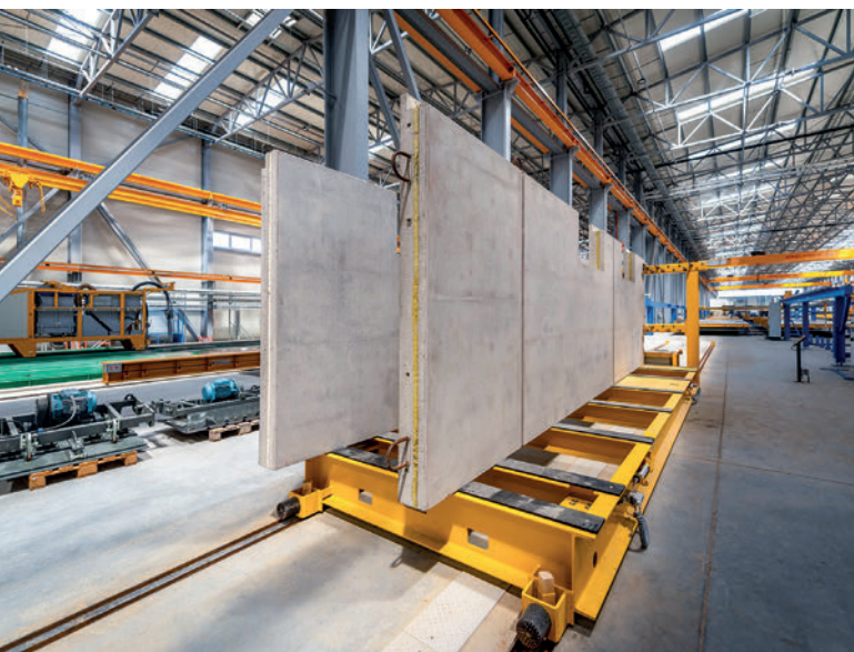
The finished prefabricated concrete walls and slabs can be produced under any weather condition and thus ensure a secure planning of the building.
