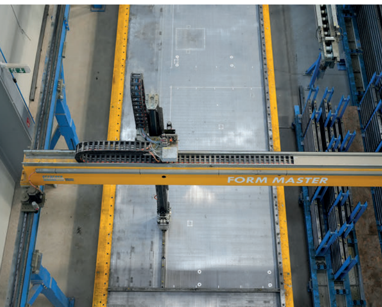
The shutters are placed exactly and automated according to the CAD planning.
