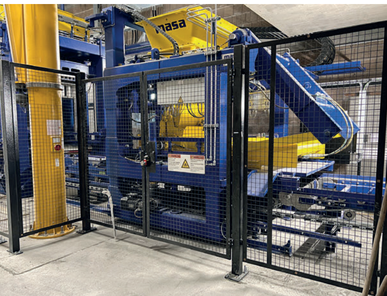
Masa XL 9.1 with column-mounted slewing grab
