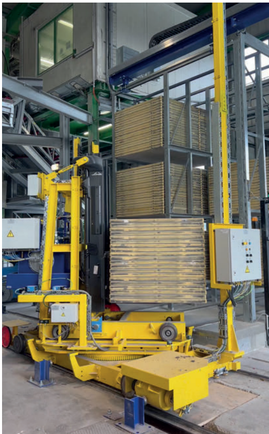
The new transport carriage with turning device and telescopic mast reliably takes over the storage and retrieval of production boards
