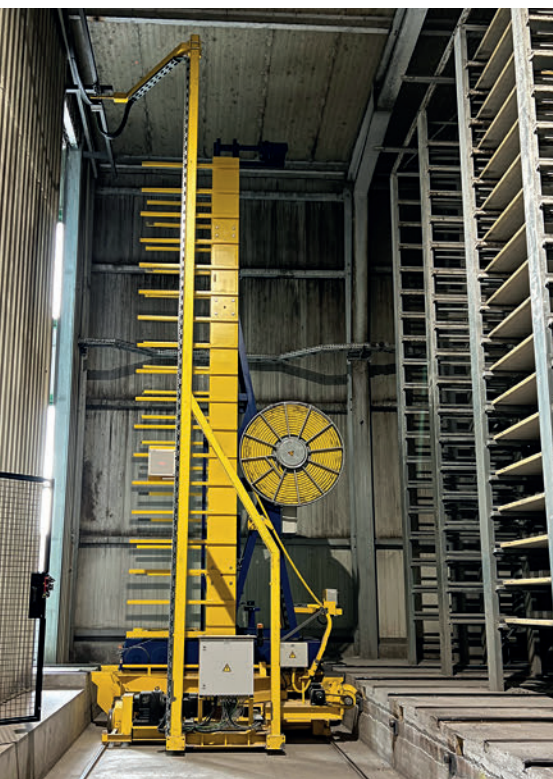
Finger car in the curing area
