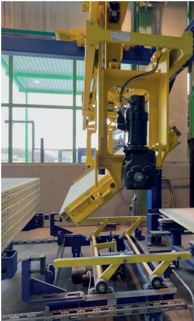
Shifter unit with vertical turning gear for individually adjustable handling of production boards
