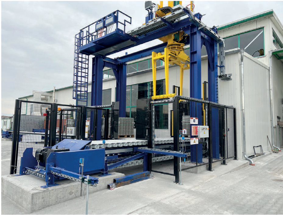
The cube shifter grabs the finished cubes with a special clamp and positions them
