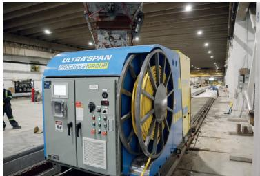
Given the challenges, Multicrete identified UltraSpan's EXT Series Extruder as the perfect solution and promptly acquired it along with ancillary machinery for the complete hollow core plant.
