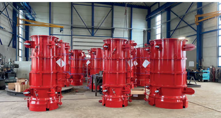
Various radial press RP outer moulds for the manufacture of concrete pipes
