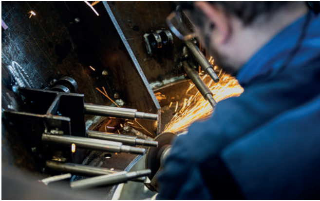
Conical Tornado core during machining
