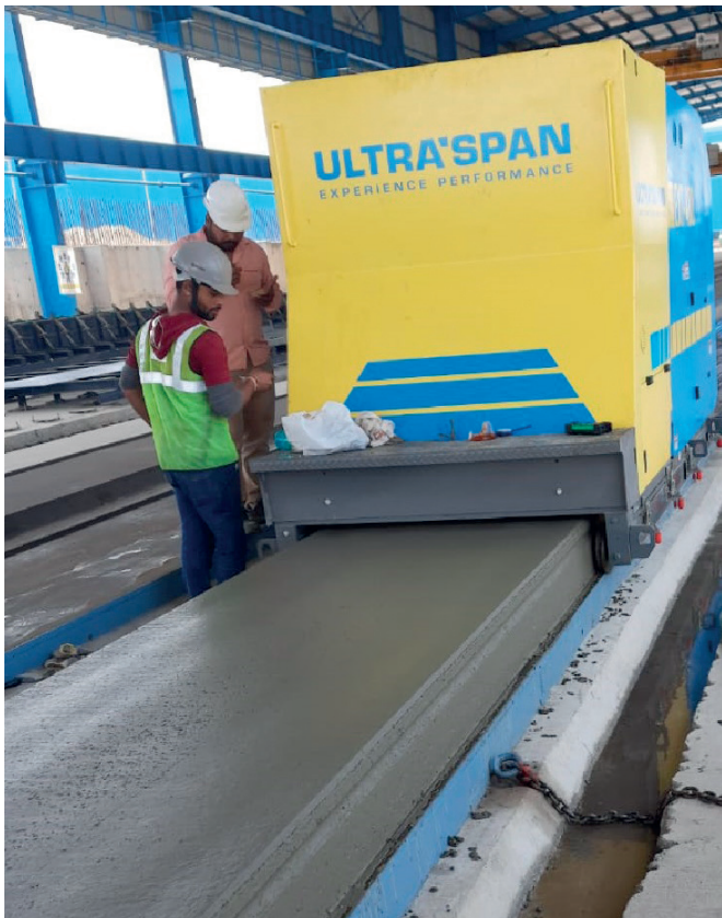
The extruder from UltraSpan is providing fast and high quality production on beds of hollow core slabs.
