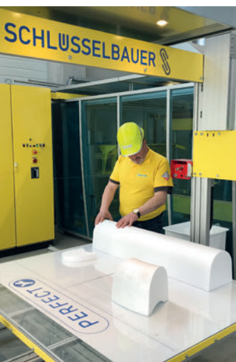
Complete channels are manufactured by means of simple cutting and gluing.
