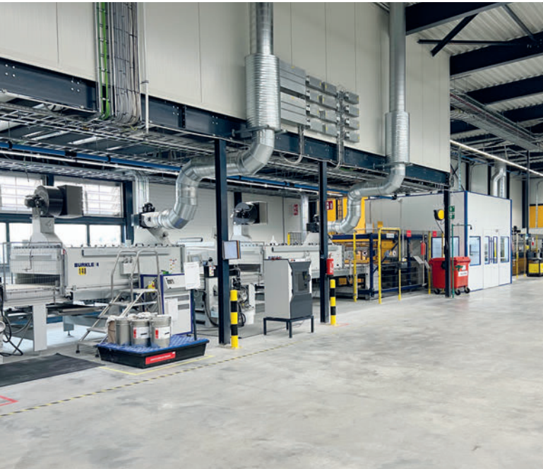
The printer prints the individual desired motifs on the products at an 8 m/min throughput speed.
