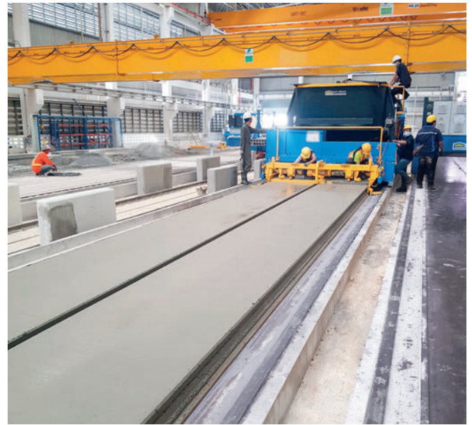
The Slipformer S-Liner® is a flexible machine. It is capable of producing 1 slab of 1.2m in width and 2 slabs of 0.6m or two slabs of 1.2m at the same time.
