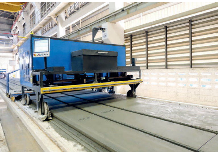
The automatic plotter SmartJet is working with the CAD data which is imported in the Ebos HC software. This machine ensures a fast marking on the slabs and no mistakes are made. The markings for the line detection are made simultaneously.
