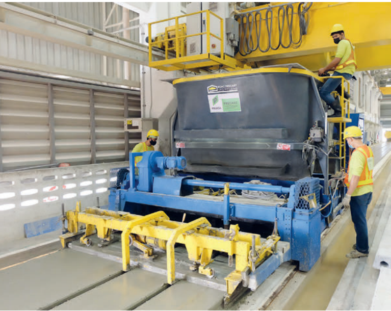
The Slipformer S-Liner® is a flexible machine. It is capable of producing 1 slab of 1.2m in width and 2 slabs of 0.6m or two slabs of 1.2m at the same time.
