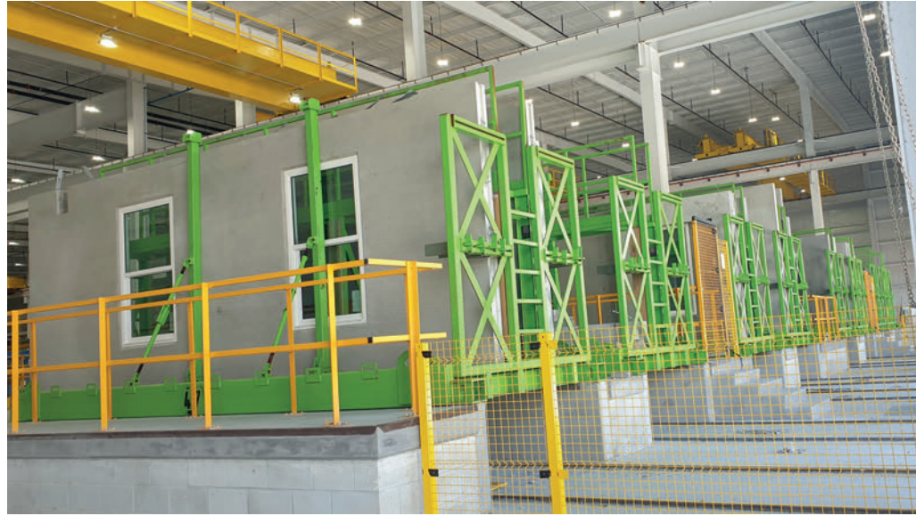
The finished walls are transported out of the hall on commissioned wall transport racks by an automatic exit system.
