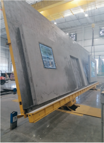
The finished walls are transported out of the hall on commissioned wall transport racks by an automatic exit system.
