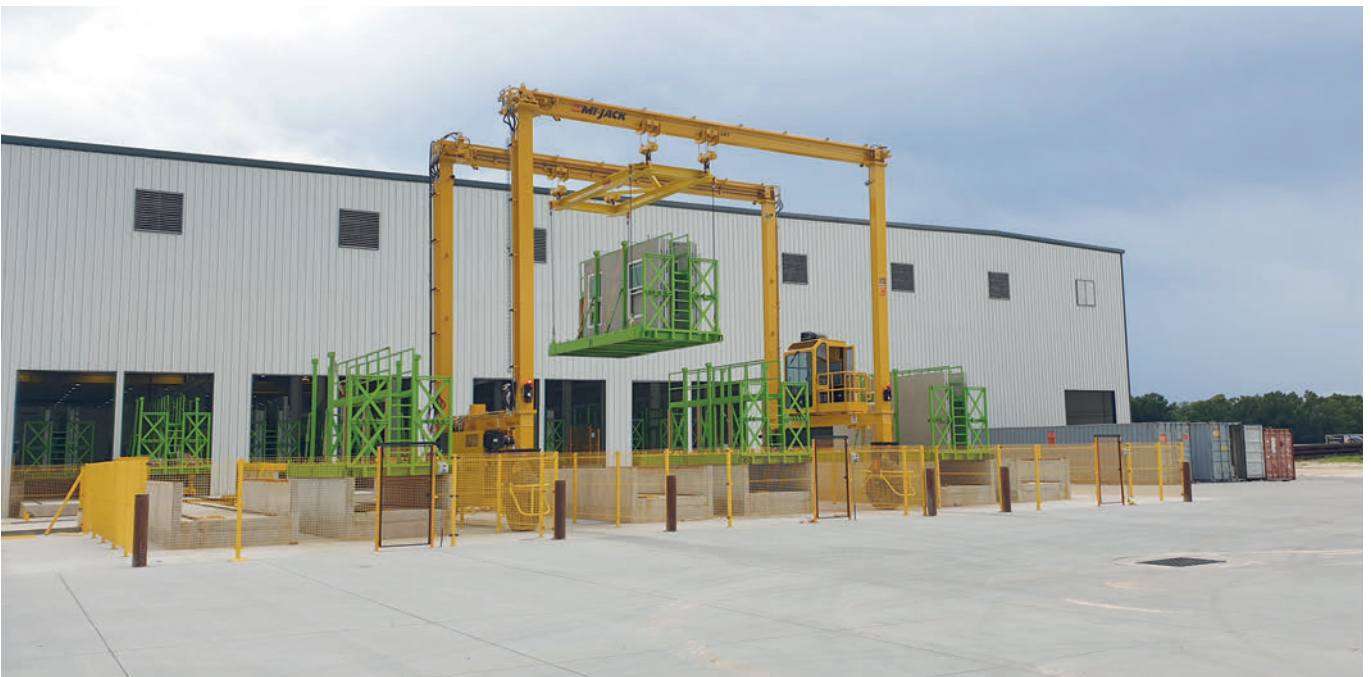
Handling in the outdoor area is carried out by a mobile gantry crane, which moves the wall transport racks in and out of storages.
