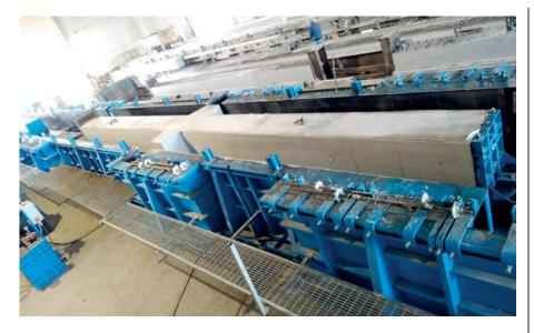
The produced pillars with corbels are 28, 5 meters long.
