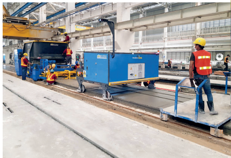
The automatic plotter SmartJet is working with the CAD data which is imported in the Ebos HC software. This machine ensures a fast marking on the slabs and no mistakes are made. The markings for the line detection are made simultaneously.
