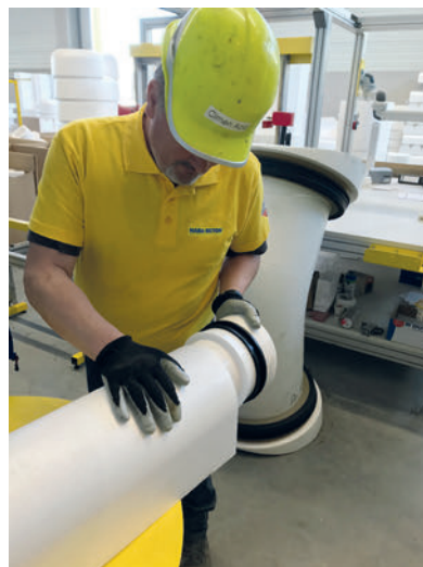
Complete channels are manufactured by means of simple cutting and gluing.
