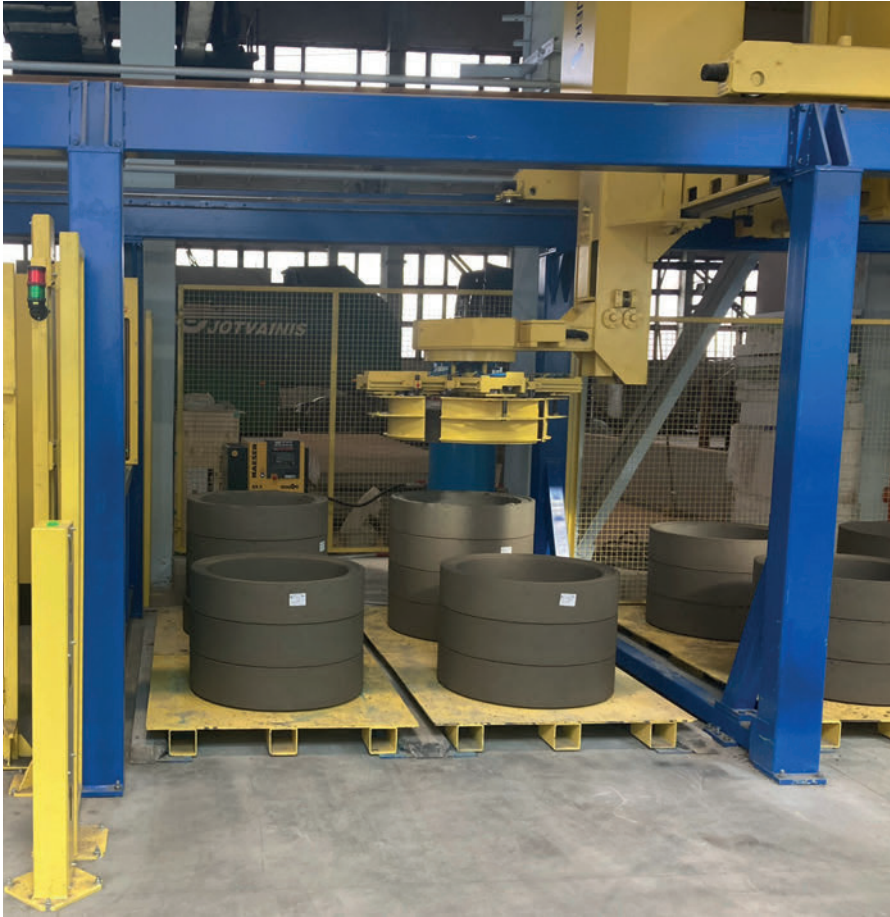
Fully automated adjustment ring manufacture and handling with automatic Ringmaster stacker.
