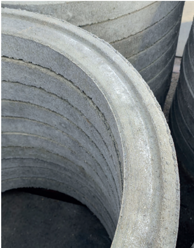
Production of adjustment rings with rebated joints without bottom pallets.
