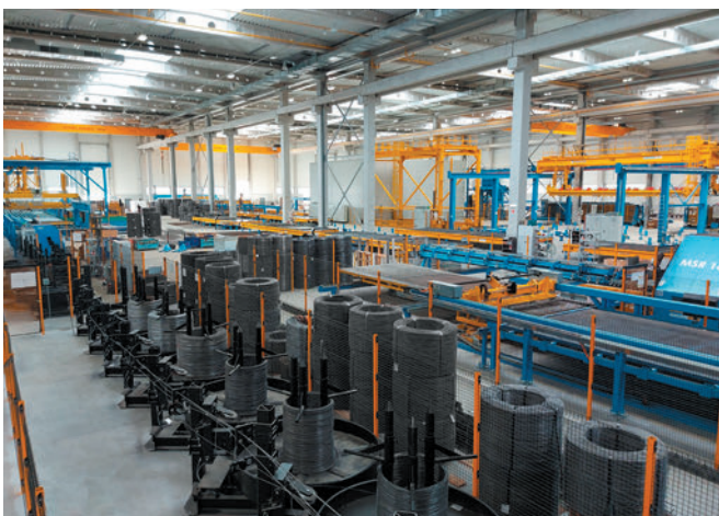
The automated plant has machinery for the reinforcement production integrated, so everything needed for the production of the concrete elements is produced in the factory itself.
