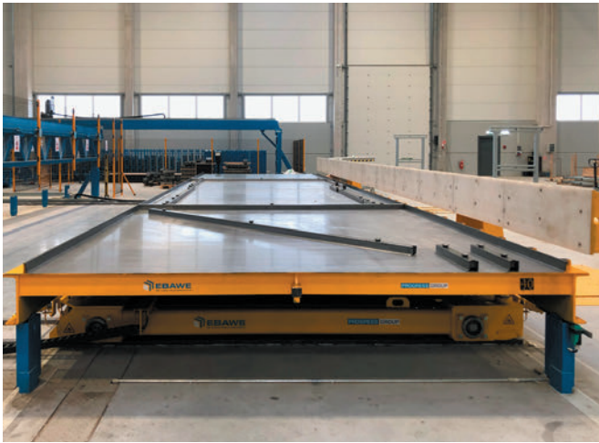
The shutters are placed exactly where they are needed in the element according to the plan - fully automated and within a short amount of time.
