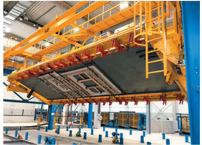
The turning equipment from Ebawe Anlagentechnik is fully automated and working precisely to the millimetre.
