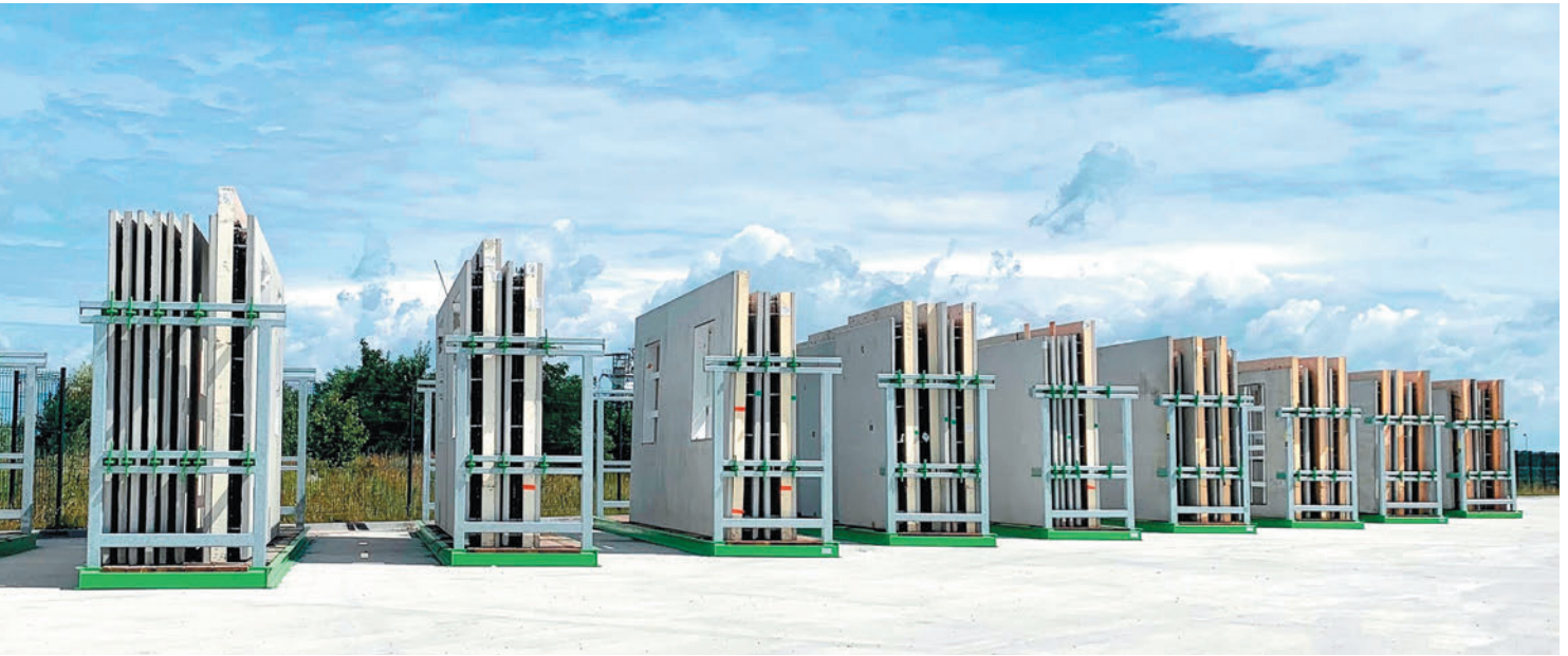
MojDom delivers prefabricated elements with the included cut outs already implemented.
