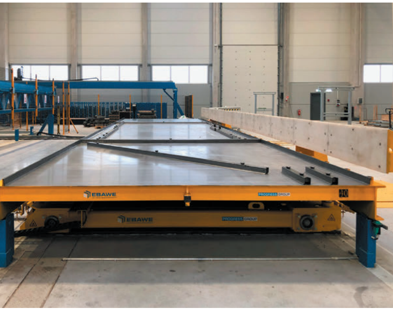
The shutters are placed exactly where they are needed in the element according to the plan - fully automated and within a short amount of time.
