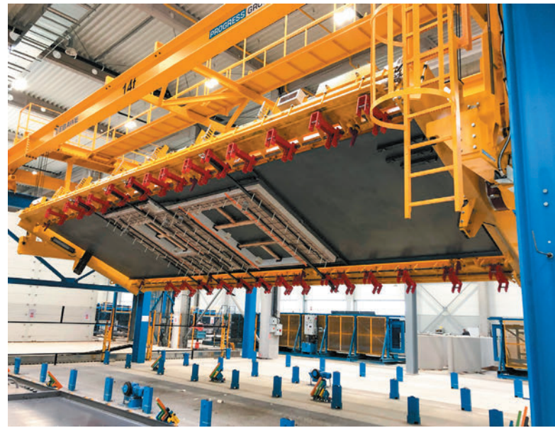
The turning equipment from Ebawe Anlagentechnik is fully automated and working precisely to the millimetre.
