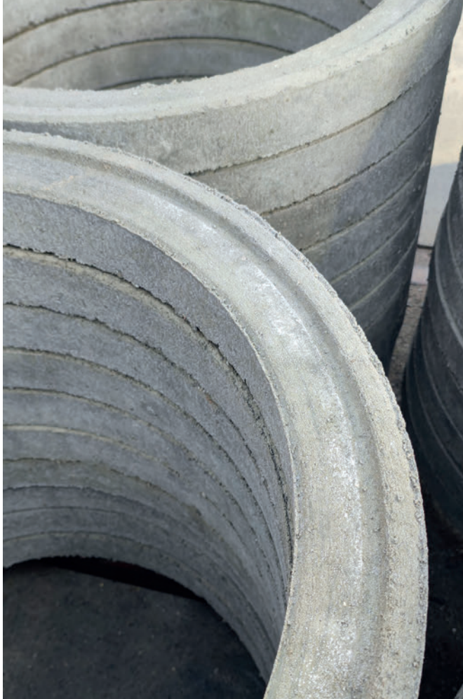
Production of adjustment rings with rebated joints without bottom pallets.
