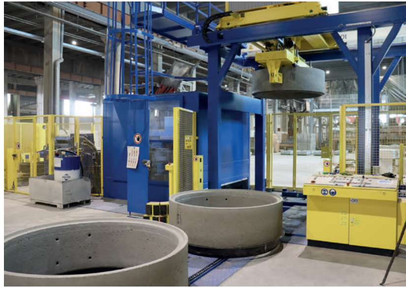
View of the palletizing station of adjoining, blue enclosed cleaning system and following pallet oiling station
