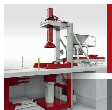
TORNADO – a global brand for manhole precast concrete elements production
